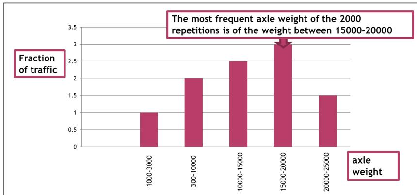
Figure 13. Example of the results of WIM survey and load spectra *Concept*
