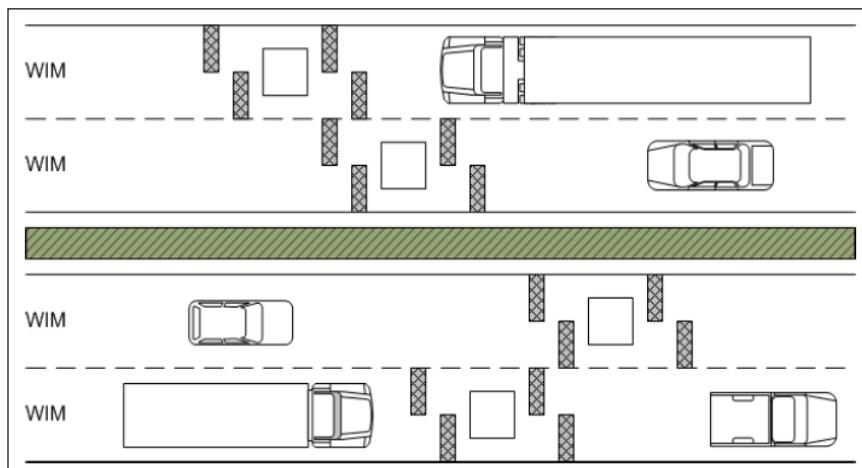
Figure 12. WIM system setup
