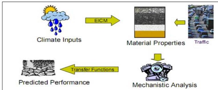
Figure 1. The Stages of MEPDG Procedure
